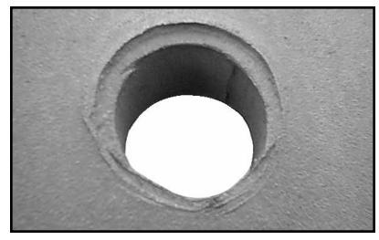
jammed blade will break either from fatigue or from catastrophic occurrence and will allow the blade to be ejected. A blade carrier damaged in this manner must be taken out of service immediately. Repair the blade carrier (contact Brown Mfg. Corp. for instructions) and replace the blades and blade bolts before returning the machine to service.
